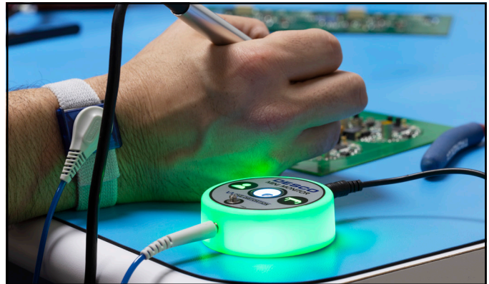
Figure 9. Illuminating green to indicate a proper operator path-to-ground
