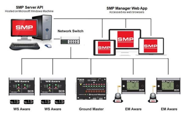
All monitoring devices are connected to a local area network with a server (physical or virtual) running the software. In general, SMP offers a flexible architecture with loosely coupled components.
